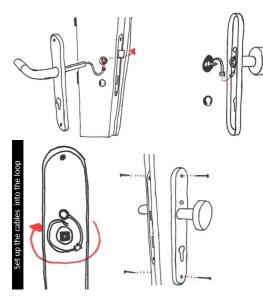
**Important:** Secure enough space for the wires and check the sharp edges on the ball side of the door.
